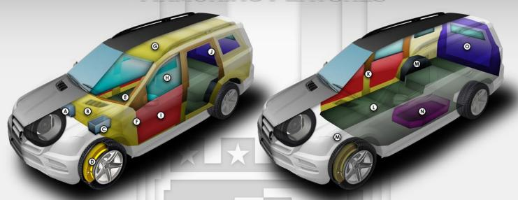
\*\* These schematics represent typical armoring of an SUV. The final vehicle (Chevrolet Suburban 3500HD) may vary depending on the client's required specifications. \*\*
