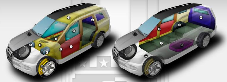
\*\* These schematics represent typical armoring of an SUV. The final vehicle (Range Rover Autobiography) may vary depending on the client's required specifications. \*\*
